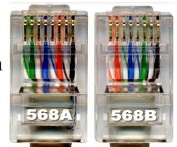
Controller and offline master controller and switch these three devices between each other using a crossover cable is better , One head is 568B, the other head is 568A. Above any equipment and computer room with a straight line , that is both 568B or 568A , Do not define the order of the straight line.
